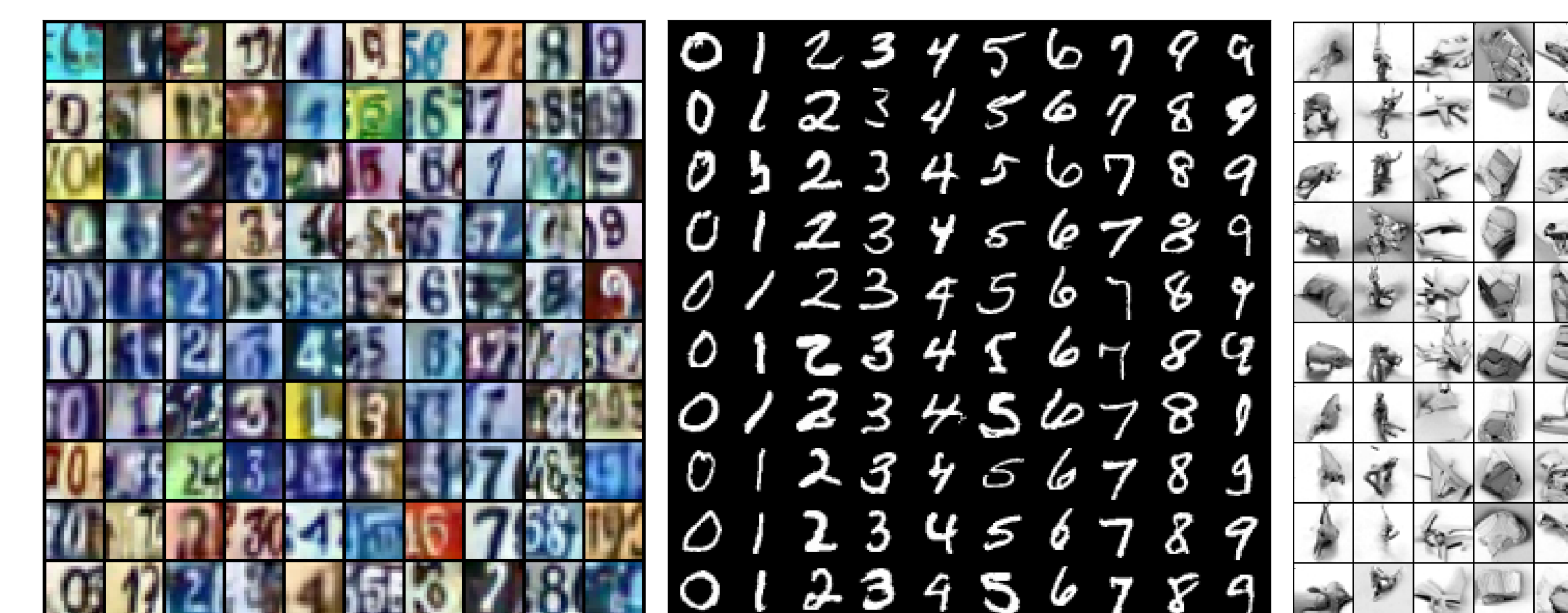
Conditional samples of the semi-supervised PixelGAN autoencoder (a) SVHN (1000 labels) (b) MNIST (100 labels) (c) NORB (1000 labels)
